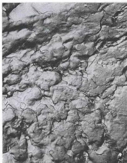
FIG. 11(b), (c). Electron fractographs of 90% Sn-bal Bi specimens which had fractured at (b) 1.55 \times 10^8 N/m 2 and (c) 8.2 \times 10^8 N/m 2 showing a dimpled structure typical of ductile fracture. 3000 \times .
